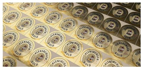
The label finishing was carried out by the **Ellerhold** printing company using KURZ ECOFIN®. The <u>cold-transfer decoration</u> impresses with brilliant printing results on a thin 10  $\mu$ m transfer carrier (formerly 12  $\mu$ m), which now uses **17 percent less material** and can save on roll changes by increasing the roll running meters. Printing is done on white, slightly textured paper instead of the
