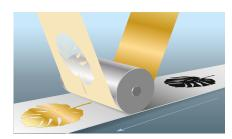
Flat digital metallization for sheet-fed involves transferring a toner-preprinted image onto paper or cardboard using a digital heat transfer process. The metallization is applied via transfer on toner before digital color printing, allowing for easy overprinting. This technology produces precise and vibrant metallic effects on printed materials.
